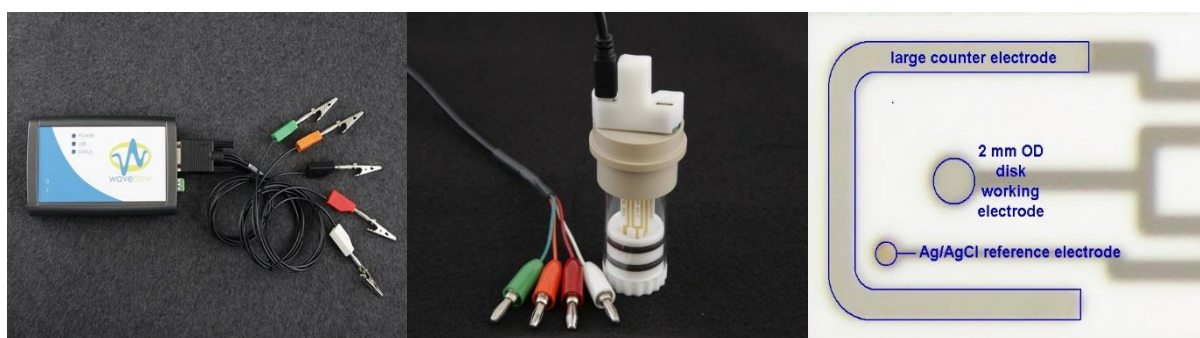
Figure 83: Potentiostat and galvanostat system WaveNowXV ® of Pine Research (left), low volume glass cell with a PTFE insert and a ceramic screen-printed electrode (middle), and a close-up of the electrode (right). Copyright 2023 Pine Research Instrumentation. Reprinted with permission.
