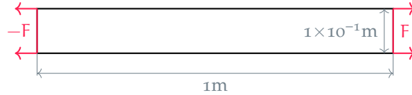
Figure 5.5: Two-dimensional bar for comparing the peridynamics material model to linear elasticity. The bar is stretched by a force F applied on both sides, going from a linear response to softening in the peridynamics model for increased load.
