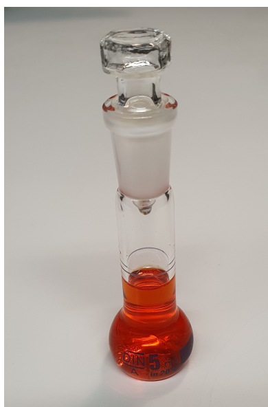
Figure 6.5.: Solution of \text{Ni}(\text{dppe})(\text{N}_3)_2 in dichloromethane. The intense orange-red color of the complex arises from d - d excitations of the nickel center, most prominently the d_{xy} \rightarrow d_{x^2-y^2} transition.
