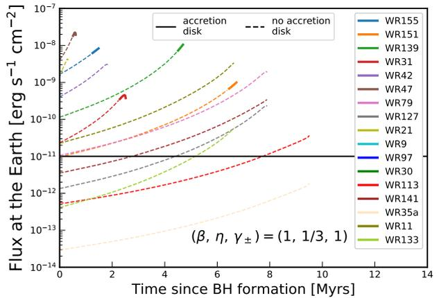
**Fig. 2.** Evolution of X-ray luminosity (*upper panel*) calculated using Eq. (11) and the corresponding X-ray flux at Earth (*lower panel*) for our BH+O models when an accretion disk can form according to our criterion (solid line). The dashed lines indicate the X-ray luminosity and flux evolution if an accretion disk could form for the entire BH+O phase. The black horizontal line shows our adopted flux detection limit.
