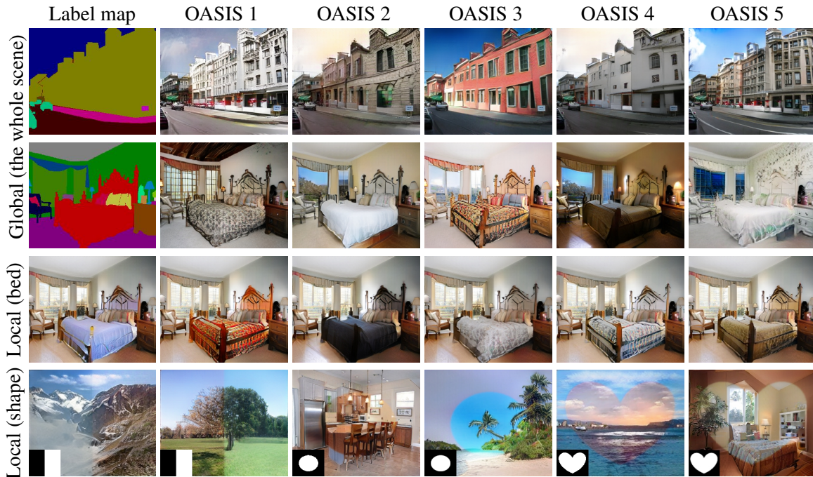
Figure 4.2: OASIS multi-modal synthesis results. 3D noise can be sampled globally (first 2 rows), changing the whole scene, or locally (last 2 rows), partially changing the image. For the latter, we sample different noise per region, like the bed segment (in red) or arbitrary areas defined by shapes.
