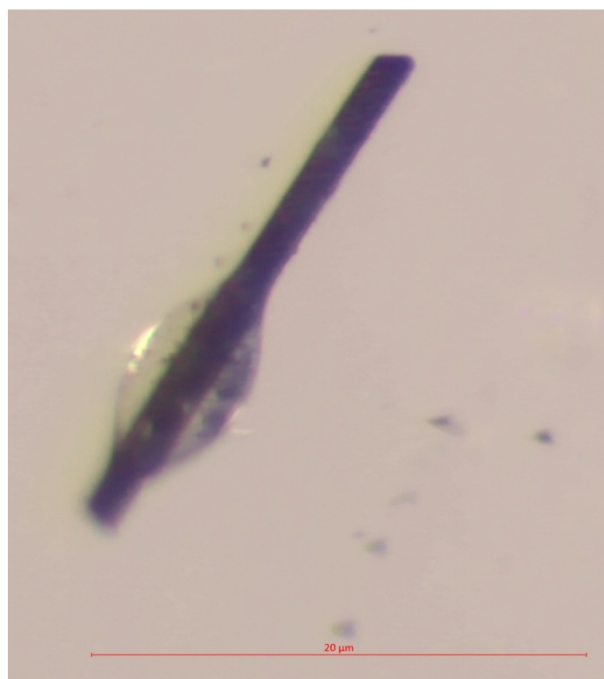
Figure 34: Image of a crystal with the composition [Sr(en) 4 ](Te 3 ) immersed in perfluorinated oil.
