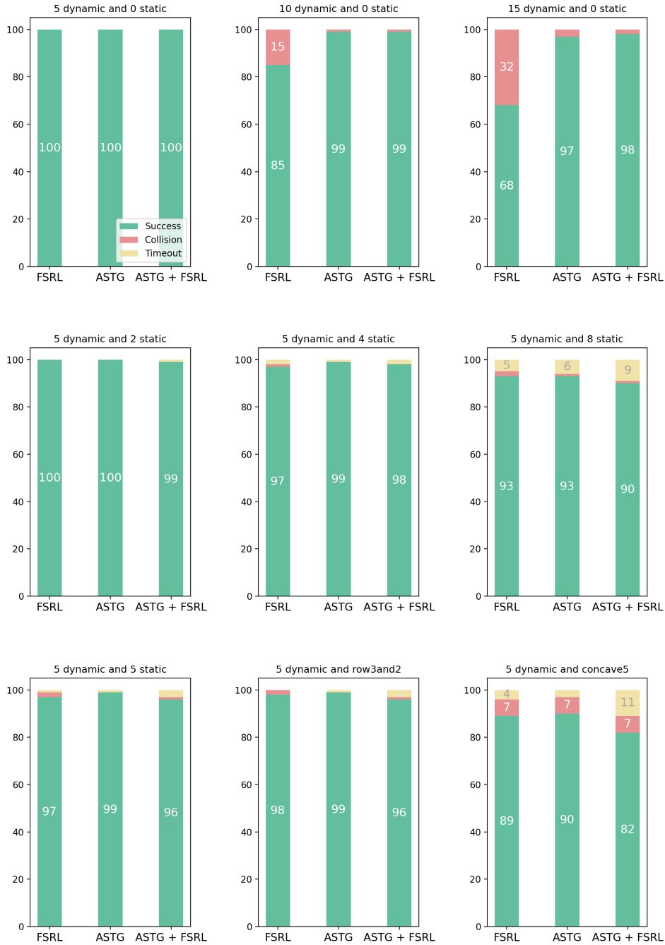
Figure 6.11: Quantative results comparison for a holonomic robot under FSRL method, ASTG method, and the combination method ASTG+FSRL.
