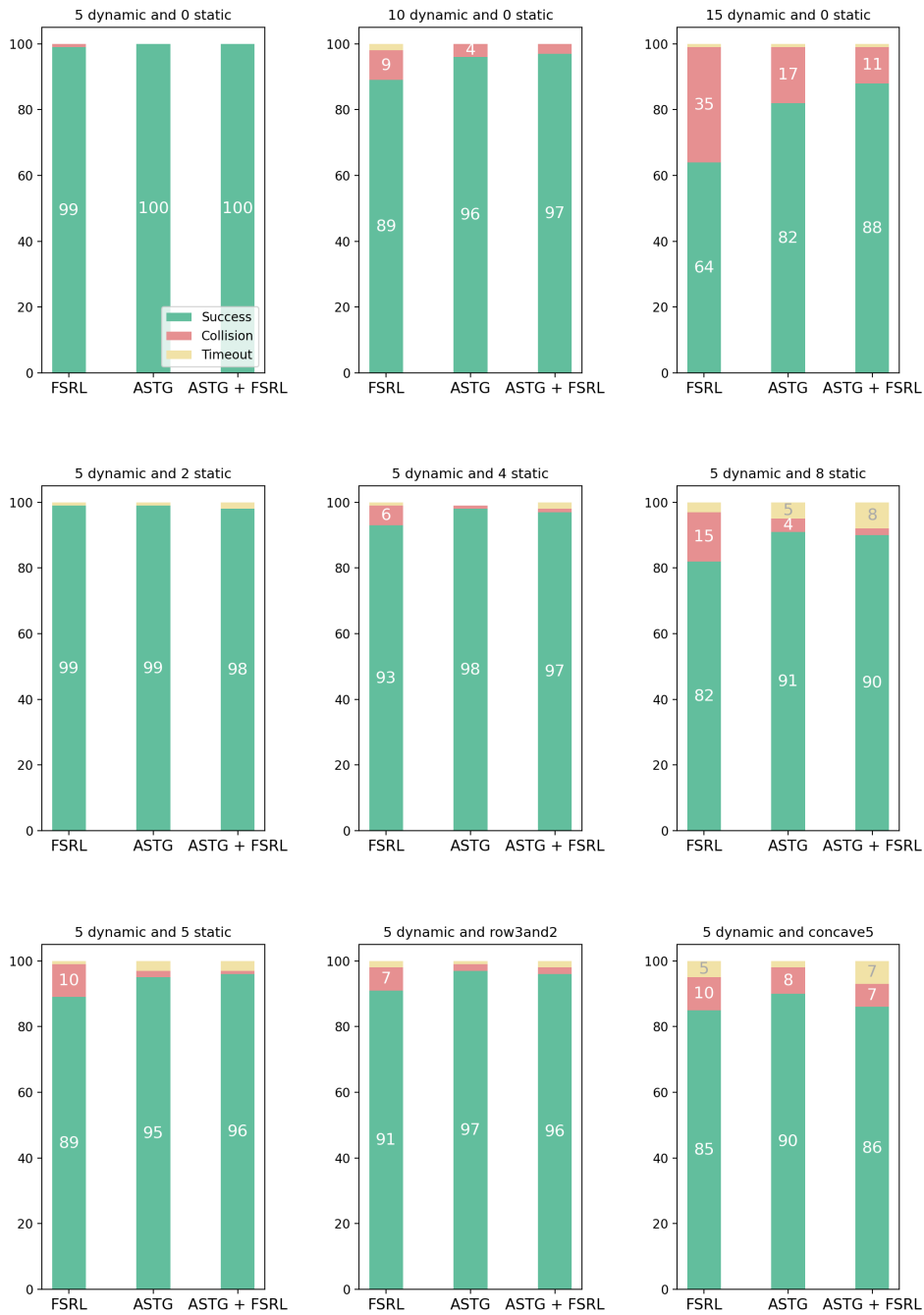
Figure 6.10: Quantative results comparison for a nonholonomic robot under FSRL method, ASTG method, and the combination method ASTG+FSRL.
