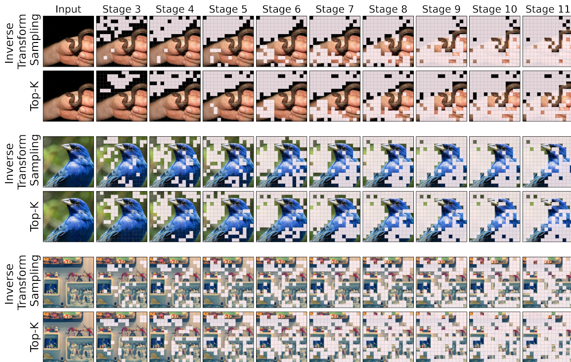
Figure 7.2: Visualization of the gradual token sampling procedure in the multi-stage DeiT-S+ATS model. As it can be seen, at each stage, those tokens that are considered to be less significant to the classification are masked and the ones that have contributed the most to the model’s prediction are sampled. We also visualize the token sampling results with Top-K selection to have a better comparison to our Inverse Transform Sampling.
