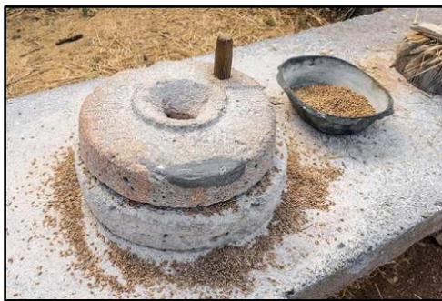
Figure 7 Manual stone-mill. Wheat grains are dropped from the top and the upper wheel is manually rotated to get flour
