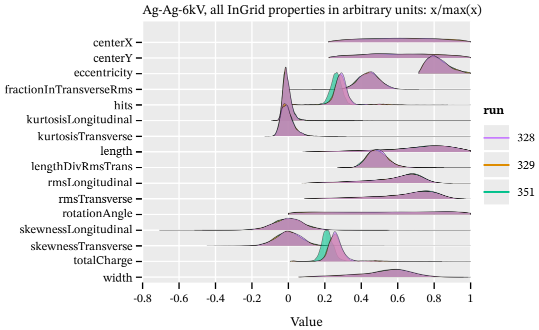
Figure H.5.: Ridgeline plot of kernel density estimations of all cluster properties split by each CDL run. Target/filter: Ag-Ag-6kV
