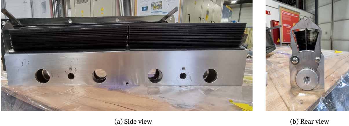
Figure 4.3.: (a): Image of the LLNL telescope outside its housing after decommissioning at CAST. Entrance side towards the magnet on the right with the largest shell radii. Both sets of mirror shells are clearly separated in the middle.(b): View of the telescope shells as seen from the detector side. Installed at CAST the telescope was rotated by about 76^\circ counter clockwise from this view. Both images courtesy of Cristina Margalejo Blasco.
