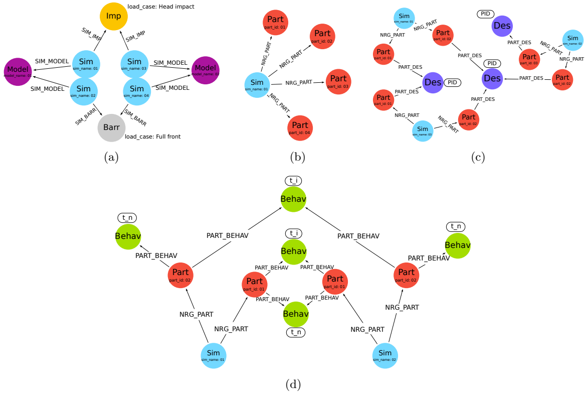
Figure 6: Illustration of the building blocks of our graph modeling. (a) A high-level simulation consists of one model and one impactor/barrier depending on the crash scenario (b). More detailed components of a simulation are the parts that are filtered as energetic parts (c), while design and (d) behavior nodes connect parts of simulations based on the similarity of the design or the crash behavior, respectively.
