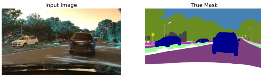
Figure 5. Input images and corresponding labels from Berkeley DeepDrive (BDD100K) dataset for the semantic segmentation task [40].
