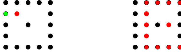
Fig. 1: Visualization of the ghost points for the forward difference in x -dimension: ghost node (red) that is used for the sparse grid forward finite differences in x -dimension in the green grid point in the left graphic, and on the right all forward difference ghost nodes that are used for the sparse grid are drawn in red.
