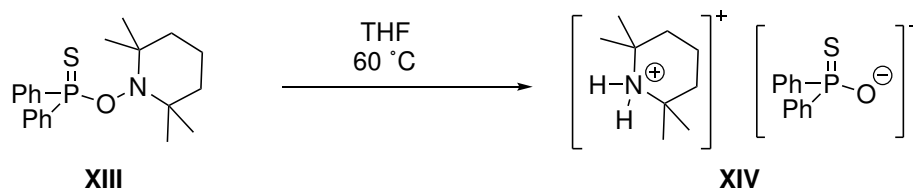
Scheme 6: Thermal N–O bond cleavage of aminoxyphosphane sulfide XIII to ammonium thiahyphosphite XIV by Heurich. 50
