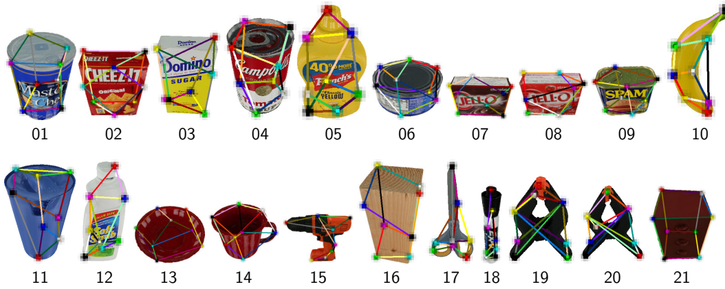
Figure 3.16: Objects of the YCB-V dataset with heatmaps of the automatically defined keypoints and their interconnections.
