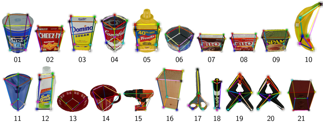
Figure 3.15: Objects of the YCB-V dataset with heatmaps of the manually defined keypoints and their interconnections.
