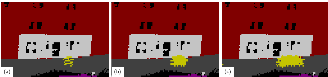
Figure 4.5: Paris-CARLA-3D dataset: Projection of dynamic persons (yellow) into the virtual OS0 LiDAR view using dataset scans from (a) only the current, (b) \pm 2 , and (c) \pm 5 adjacent positions. The foreground person is incomplete when using just a single scan (a) but significant movement artifacts appear for a larger scan window (c). We use a window of \pm 2 (b) for our experiments as a compromise between complete scans and remaining artifacts.
