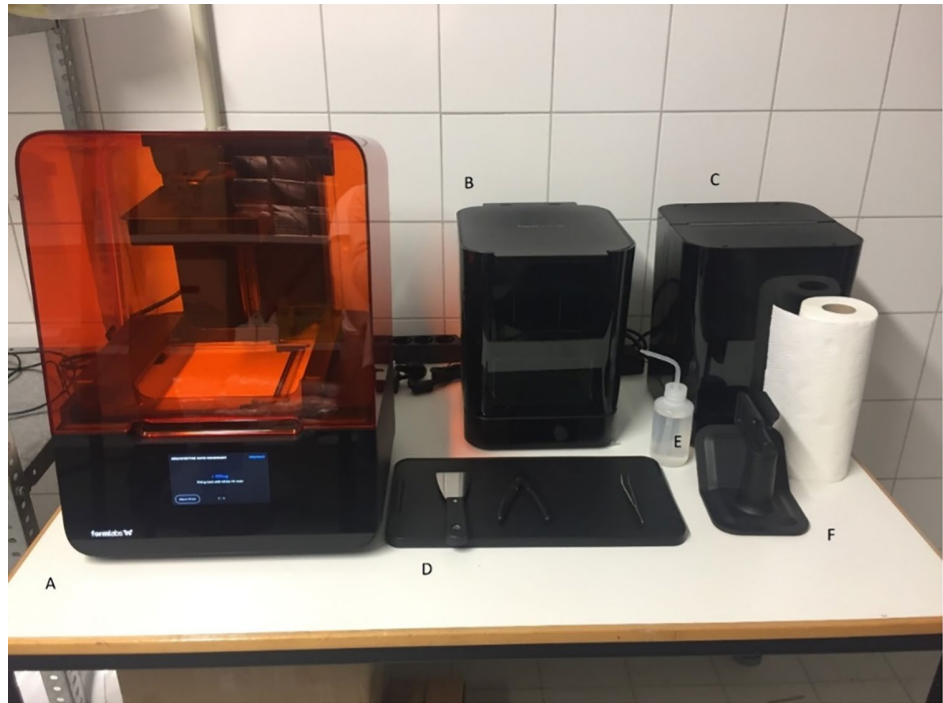
Fig. 4 Workplace setup: A 3D printer, B washing device, C curing device, D essential tools, E isopropyl alcohol for precision cleaning, F processing handle
