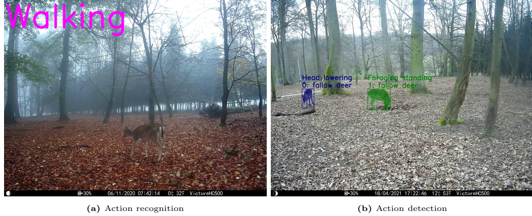
Figure 5.1: Comparison between action recognition and action detection: The action recognition (a) only classifies one action from one actor in a frame. The action class is written in the top left corner. If there are multiple actors present, the outcome would be unclear. The action detection (b) localizes each actor and describes its action. The predicted action is written above each bounding box. A classification and tracking of actors is not necessarily included in the action detection.
