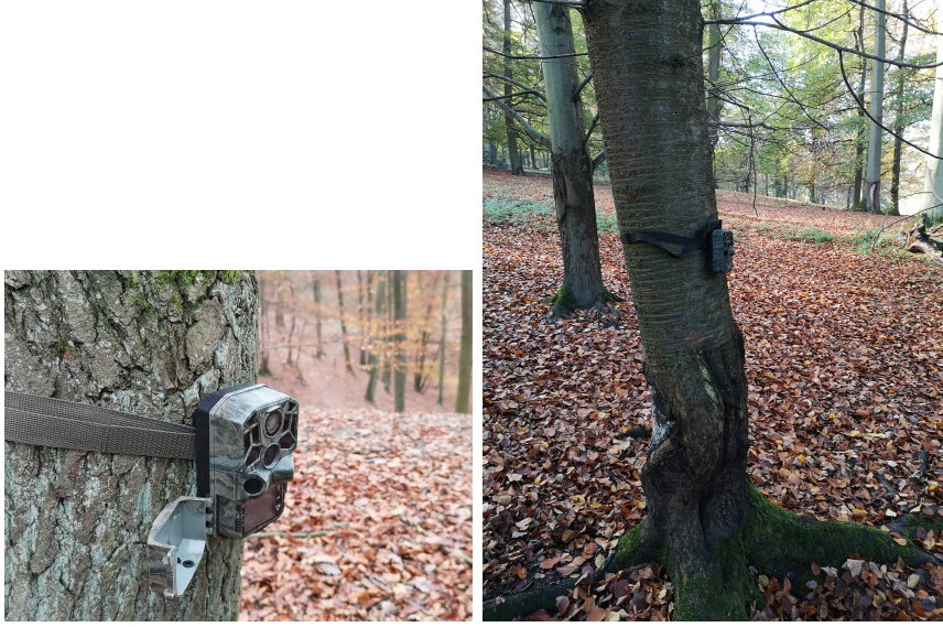
Figure 3.1: Our Victor HC500 camera traps mounted on the trees in the wildlife park Rolandseck (Germany).
