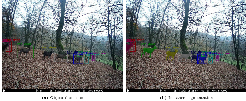
Figure 4.2: For an object detection (a) each object is localized with a bounding box. The instance segmentation (b) adds an instance mask for each object. Often both approaches include an object classification, which results in the written object class above the bounding box.
