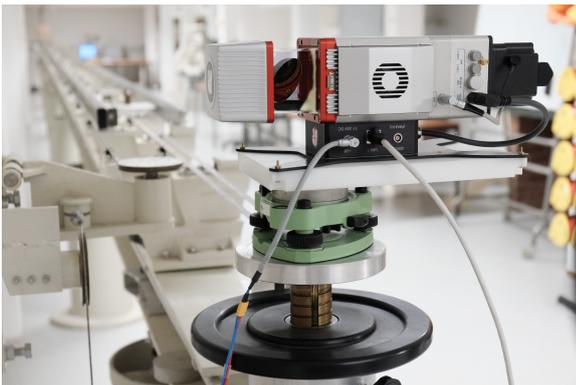
**(a)** Mounting of the 2D laser scanner RIEGL miniVUX-2UAV for measurements.
