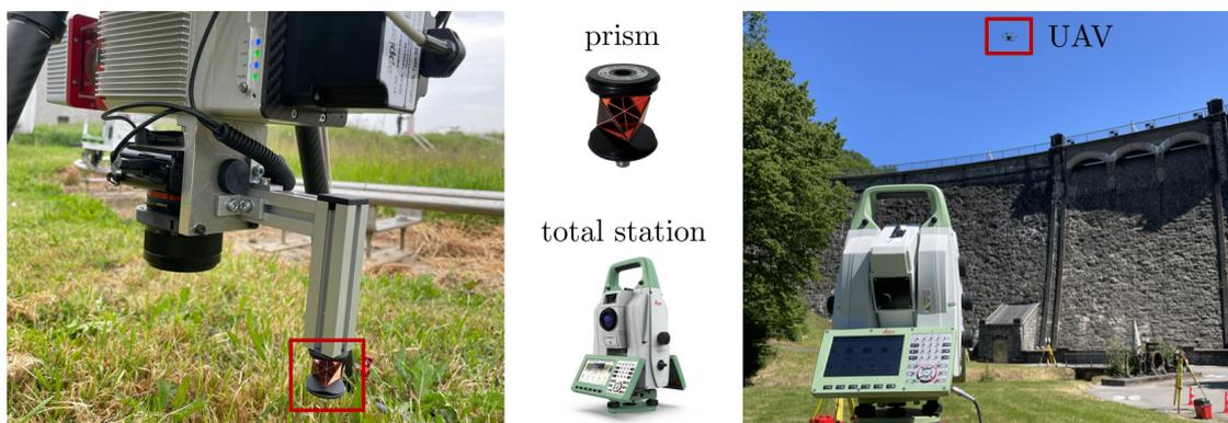
**Figure 6.1:** Scanning of a water dam with UAV-based laser scanning including the prism tracking with a total station.
