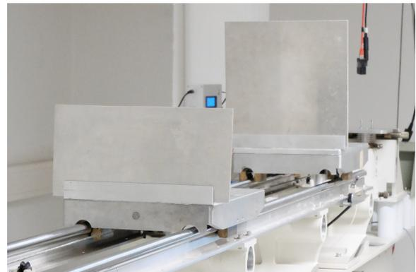
**(b)** Two aluminium targets used within the multi-target investigation.
