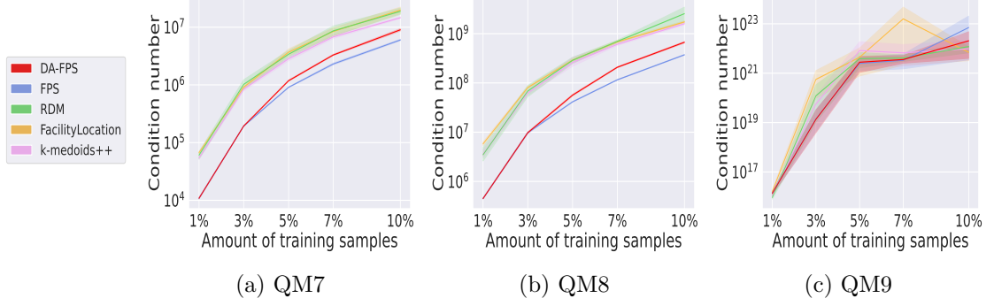
Figure B.3.: Condition number of the non-regularized Gaussian kernel obtained from the QM datasets selecting training sets of various sizes and according to different sampling strategies. The reported experiments consider the experimental setup described in Section 7.1.2. The y-axes of the graphs are on log scale and the error bands represent the confidence interval over five independent runs of the experiments. The figure extends the results illustrated in the top row of Fig. 7.3 including DA-FPS initialized with k = 100 and u = 3\% .
