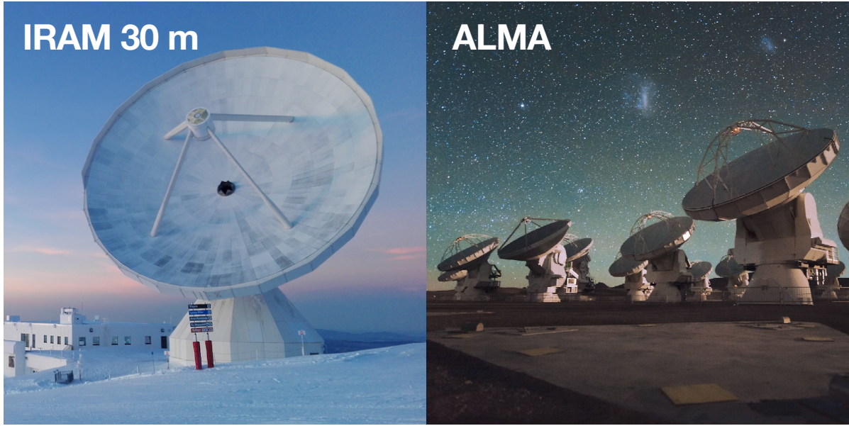
Figure 2.3: IRAM 30 m and ALMA. The left image shows the IRAM 30 m radio telescope on Pico Veleta, Spain, at an altitude of 2850 m (Image credit: IRAM/K. Zacher). The right image shows the interferometre ALMA, consisting of 66 antennas with 7 m or 12 m diameter. ALMA is located in the Atacama desert in Chile at an altitude of 5000 m (Image credit: ESO/C. Malin).
