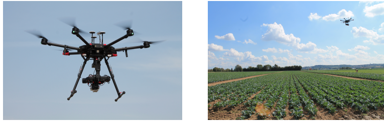
Figure 2.2: DJI Matrice 600 hexacopter for UAV image-based measurements. Image source: Kierdorf et al. [7].
