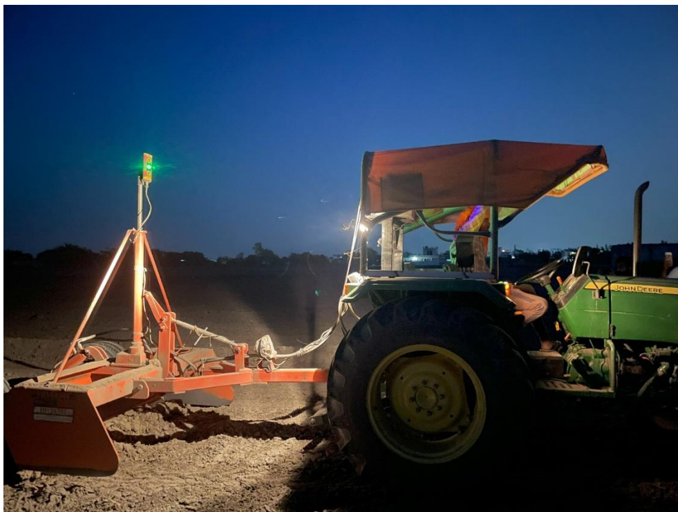
Figure 3.1: Laser land levelling technology operated at night in northwestern India, highlighting the demand for the technology
