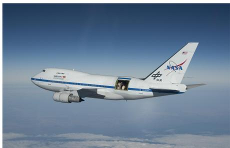
Figure 1.11: SOFIA with its telescope door open during a test flight (Credit: NASA/ Jim Ross).
