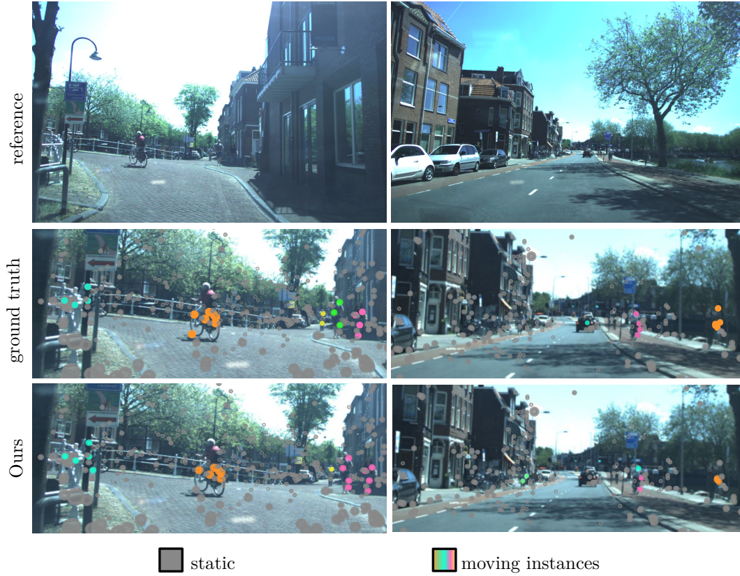
Figure 7.8: Qualitative results of our Radar Instance Transformer on the View-of-Delft validation set. The camera images are shown for reference. The ground truth instance labels and the corresponding instance predictions are projected into the reference image. The ground truth and the predictions are cropped for better visibility.
