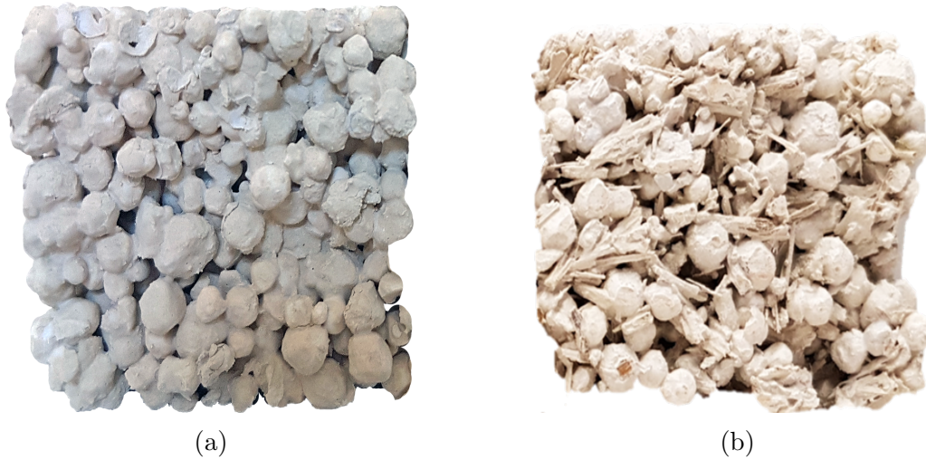
Figure 6.8: 6.8 Samples of bonded leveling compound (a) CP 0 in Binder 1; (b) CP 30 in Binder 2
