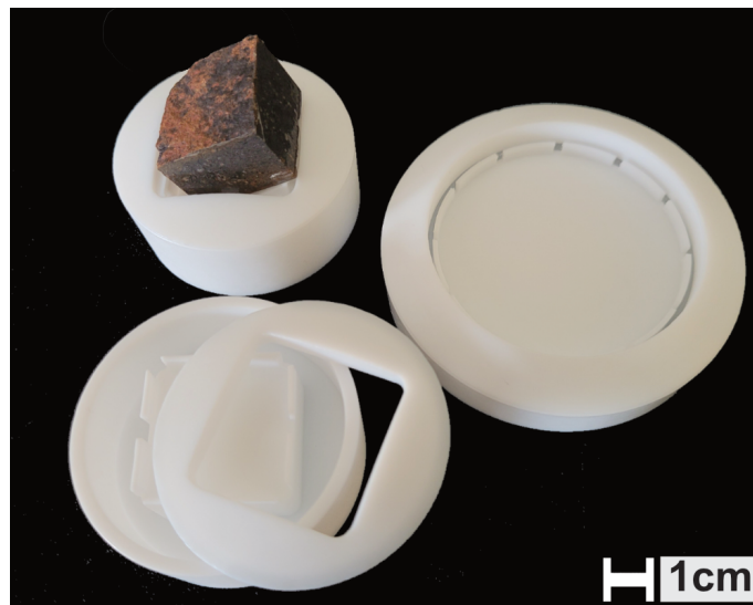
Figure 2.4: The different types of used Teflon ® containers for collecting artificial rainwater samples. All containers have a lid that is removable to ensure that only water that was in contact with the rock varnish is collected in the containers. The larger containers (right) were used for the larger samples in the climate chamber experiment and the smaller containers (left) were used for the rock cubes from the irrigation experiment. One of the rock cubes with an angle of 30° can be seen on the top left side.
