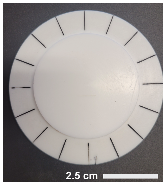
Figure 2.1: The Teflon ® plate that was used for the colour measurements. The marks on the outer ring were used to turn the chroma meter by the same angle during every measurement.
