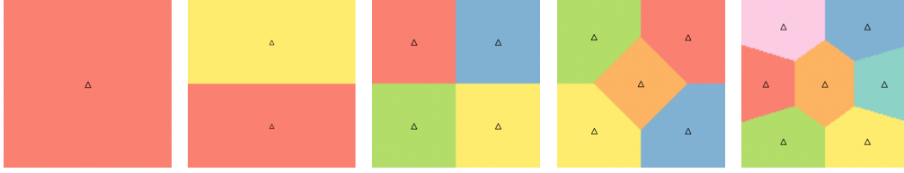
Figure 5.7: Plot of the Lloyd's centroidal power diagrams for n = 1, 2, 4, 5, 7 cells from left to right. The sites coincide with the barycenters of the cells.
