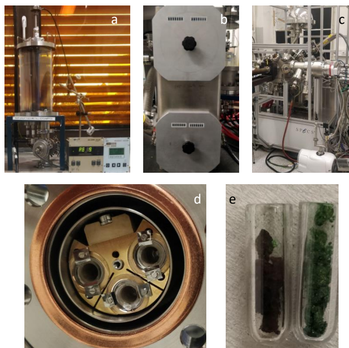
Figure 29: Experimental setups used for the PVD experiments performed with PyrSQ-C1 in the Resel group. a) set up of evaporator 1, b) evaporator 2, c) evaporator 3 (UHV PVD set-up), d) close-up on the evaporation chamber of evaporator 3, e) crucibles for evaporator 3 before (right) and after (left) PVD experiments.
