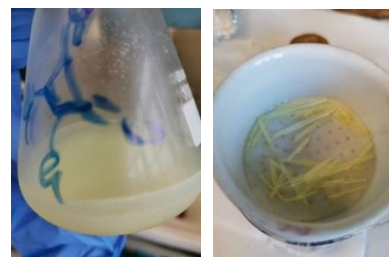
Figure 8: Synthesis of 2 (besides the desired squarylium chloride 60% of non-reacted squaric acid were reisolated). Pictures on the right show the isolation of the desired product as large crystals.
