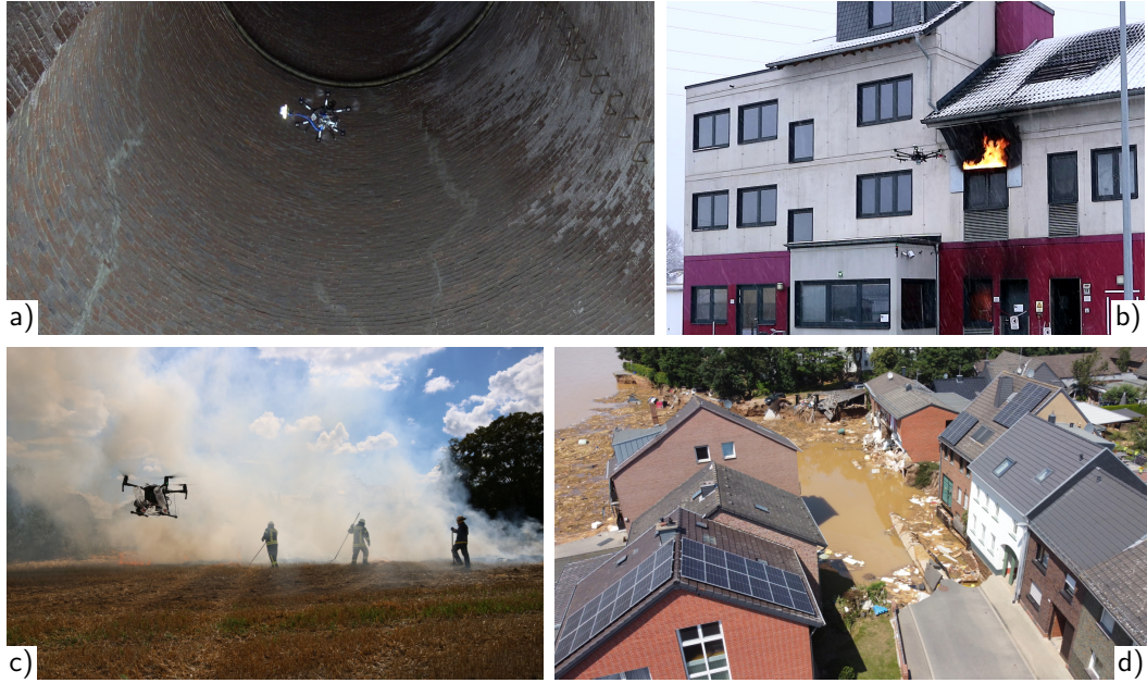
Figure 1.1: Applications: a) Industrial inspection inside a chimney. b) Targeted examination and localization of facade fires. c) Screening for clusters of embers during wildfire exercise. d) Exploration during a natural disaster without endangering first responders.
