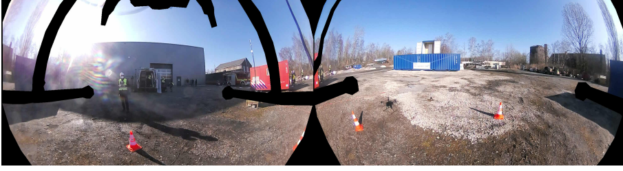
Figure 2.1: Camera distortion: straight edges in 3D appear as curved lines in the image. The curvature typically increases with distance to the image center.
