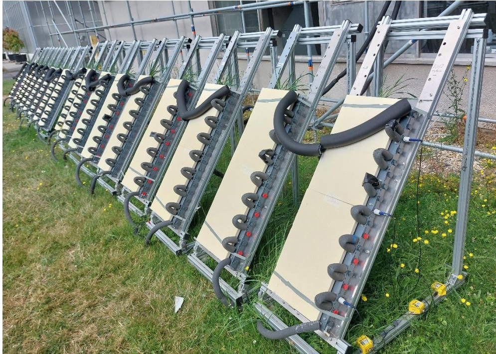
Figure E.1 Custom-made rhizotrons with passive and active temperature regulation.
