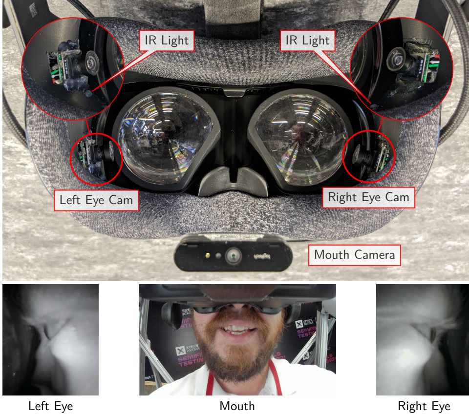
Figure 2.2: The modified Valve Index VR headset. We attached three additional cameras to capture the eyes and the mouth expression of the operator. The inside of the VR headset is lit using IR LEDs. We show the corresponding camera views at the bottom.
