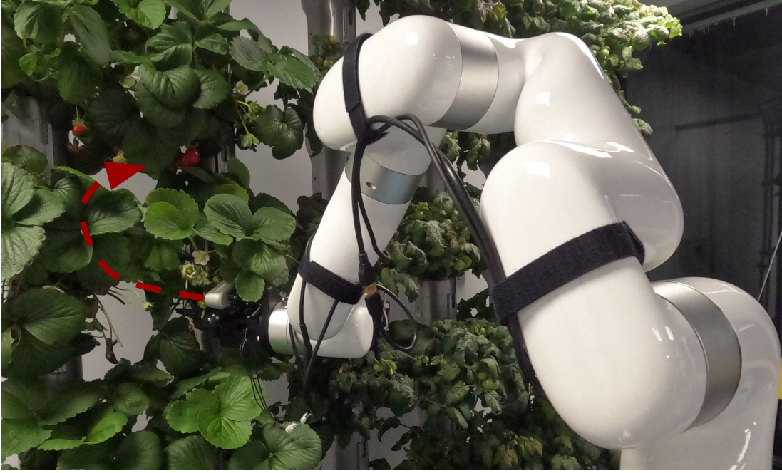
Figure 1.1: Active perception enables a robot to actively decide where to collect informative measurements. This is relevant for achieving robot autonomy in unknown environments, as no prior knowledge is available and robots need to adapt their perception strategies on the fly based on the information in the acquired measurements. For instance, to inspect or pick fruits, a robot arm needs to actively reposition its onboard camera to better perceive the target fruit and avoid occlusions, such as by following a path indicated by the dashed line. Image adapted from Federico Magistri.
