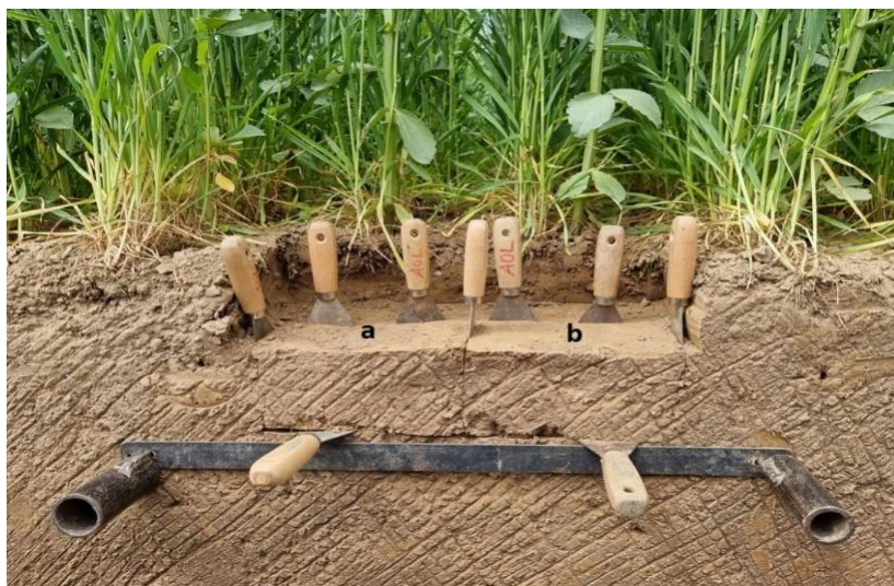
Figure S4.3: Monolith of size 20 cm (length), 10 cm (width) and 10 cm (depth) were taken at a depth of 10-20 cm, 40-50 cm, 50-60 cm and 60-70 cm. Two replicates ('a' and 'b') from each plot were taken, resulting in 8 samples per plot (2 replicates and 4 depths)
