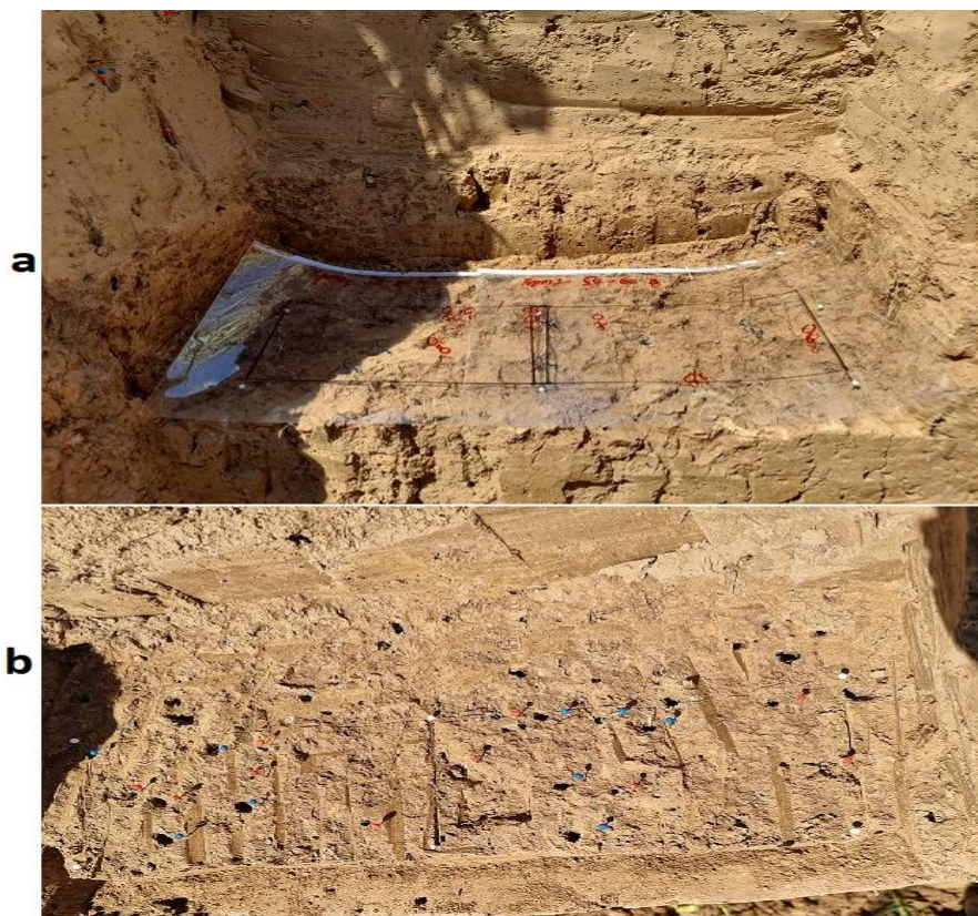
Figure S4.4: (a) The smoothed surface measuring 10 x 40 cm at a depth of 40 cm was covered with transparent plastic and labeled for the small and large biopores (2 replications of 10 x 20 cm). (b) Biopores in the soil were labeled with red (>5 mm) and blue (3-5 mm) needles representing the size of biopore.
