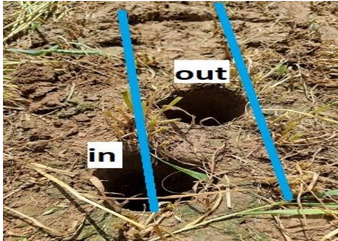
Figure 3.3: Soil core method. Position 'in' represents the samples taken from the rows in melioration area (30 cm wide), while position 'out' represents the area between two rows.
