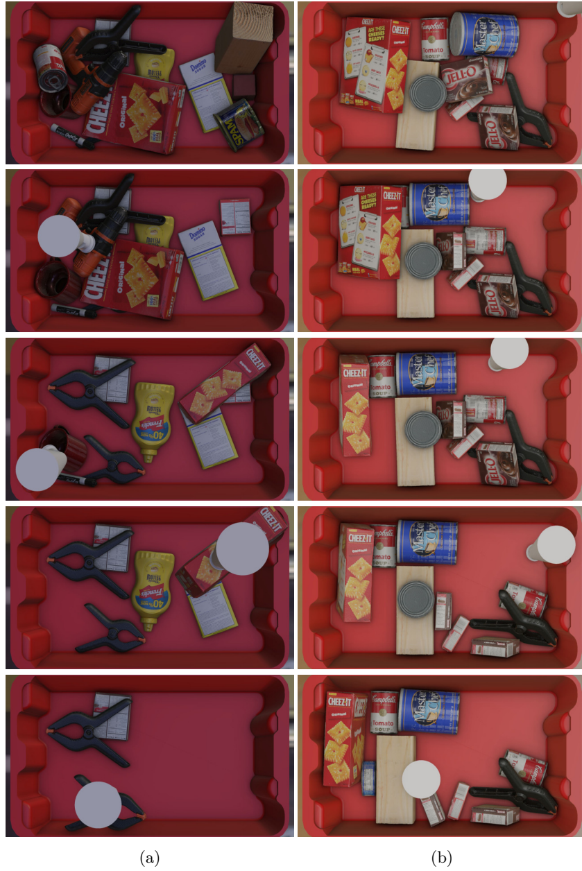
Figure 2.8: Exemplary scenes from the dataset demonstrating the evolution of the scene while the gripper is performing picking (a) and moving (b) actions. Objects in the tote are covered/uncovered as the scene evolves.
