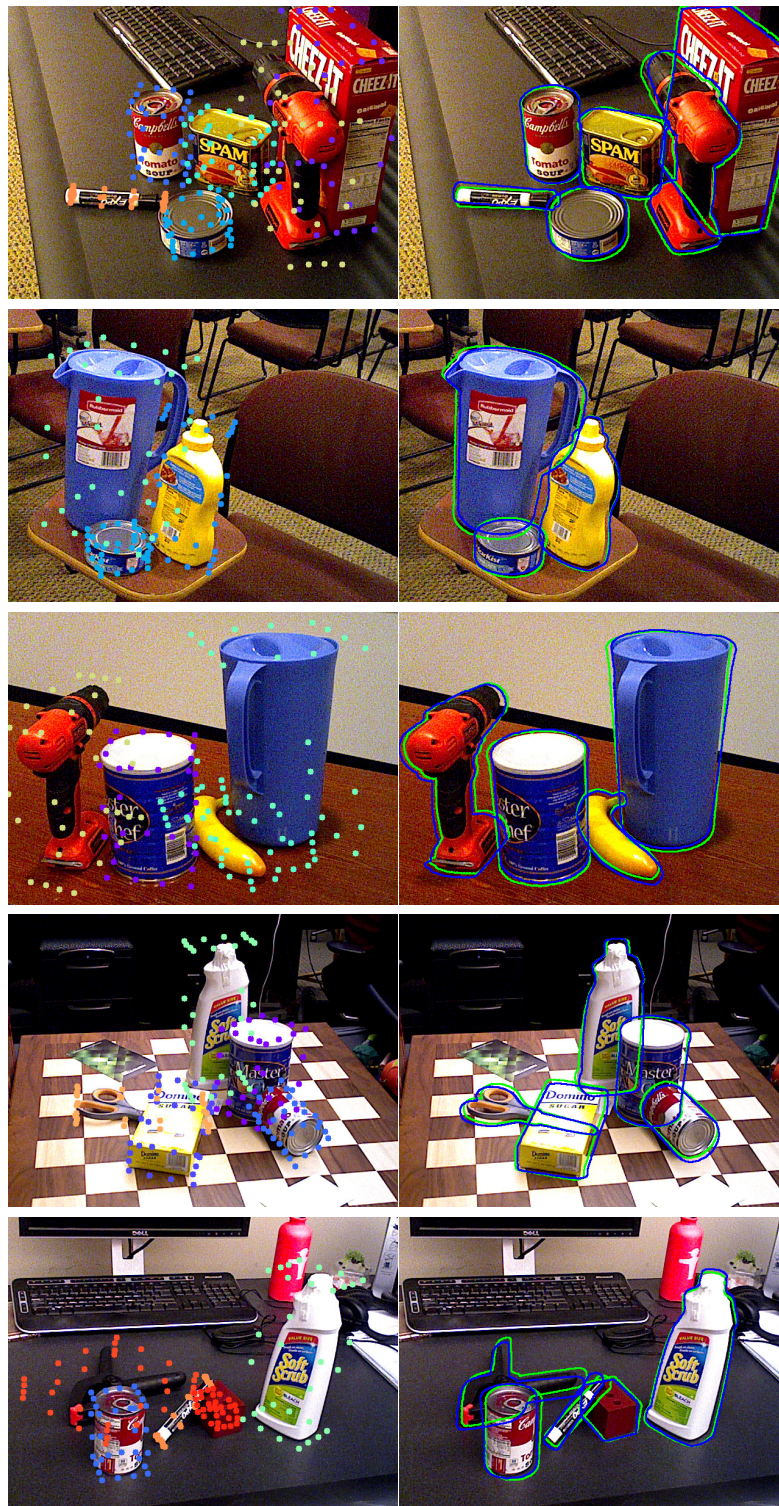
Figure 6.5: Qualitative results on YCB-Video test set. Left: The predicted IBB keypoints overlaid on the input images. Right: Ground-truth and predicted object poses are visualized as object contours in green and blue colors, respectively.
