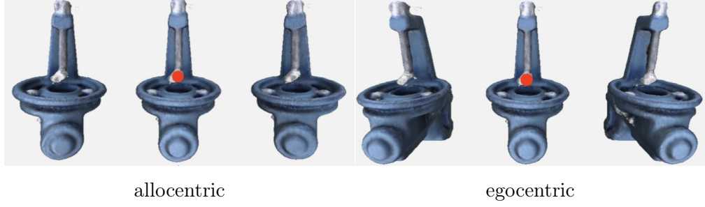
Figure 5.5: Allocentric & egocentric representations. The intersection of the camera ray with the image plane is shown using red dots. Object appears different under egocentric representation despite having the same orientation parameters due to translation lateral to the image plane. Camera intrinsics are chosen to exaggerate visual differences. This phenomenon is not observed under allocentric representation. Figure adapted from Manhardt et al. (2020).
