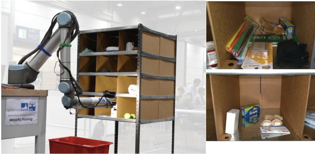
Figure 2.4: Amazon Picking Challenge (APC) setup (Schwarz et al., 2018b). Left: Amazon-Kiva Pod and the robotic arm with the RGB-D camera and the suction gripper. Right: Exemplary bin layouts.
