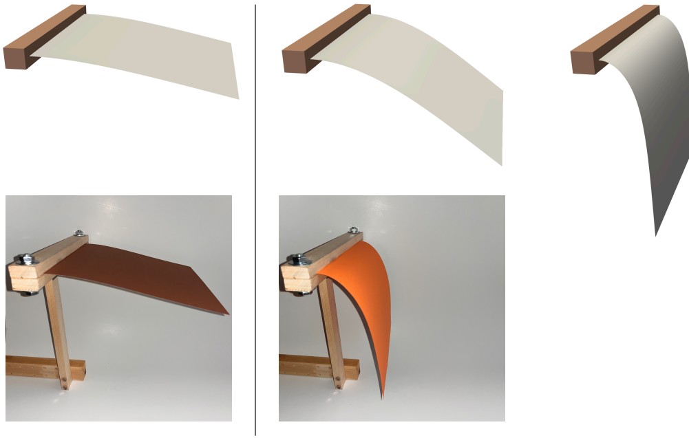
Figure 4.3: Top row: numerically computed deformed configurations of a plate, clamped on the left side, under a uniform vertical load, with homogeneous material, with Lamé constants scaled with 1.0 (left), 0.286 (middle), and 0.02 (right). Bottom row: photos of physical deformations of paper. Left: thick paper (300g/m 2 ) glued on thinner paper (120g/m 2 ). Middle: only thin paper (120g/m 2 ).
