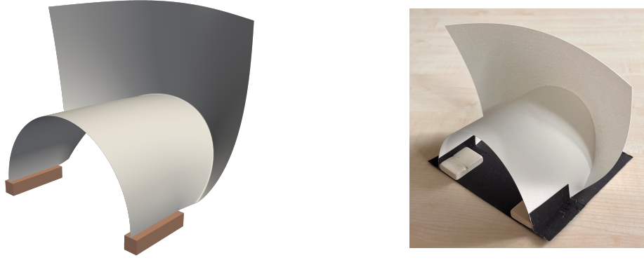
Figure 5.4: Left: Computed deformation of a thin plate with a single arc as fold curve. Right: Picture of a sheet of paper folded along the arc curve \Sigma .
