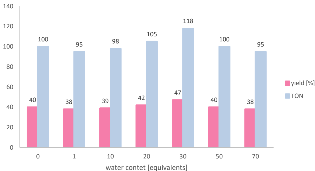
Figure 74: Results of the cobalt-catalysed cyclopropanation with different water content.
