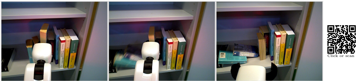
Figure 4.2: Sample sequence of the robot causing the other books on the shelf to be disturbed significantly.
