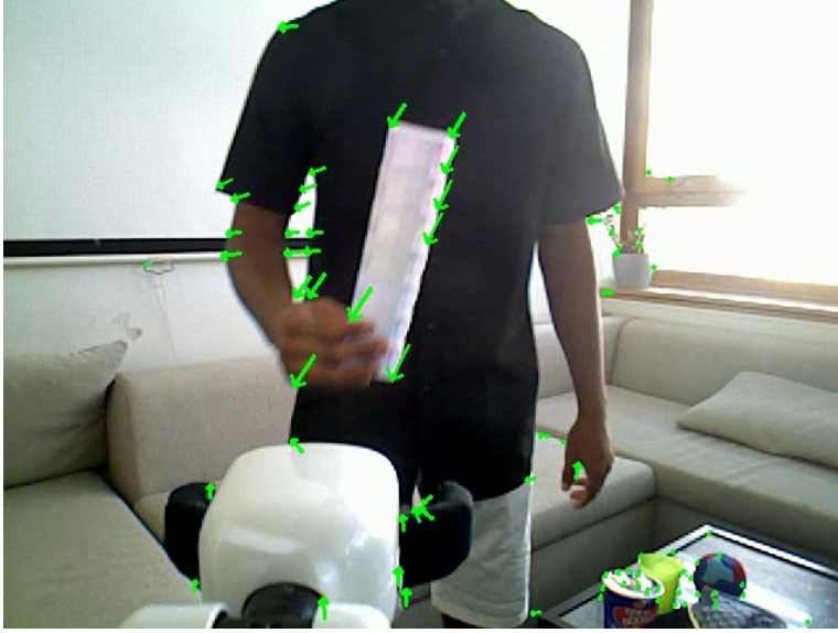
Figure 2.2: An illustration of sparse optical flow computed between two consecutive video frames. The green arrows indicate the motion of trackable corner points in the image.
