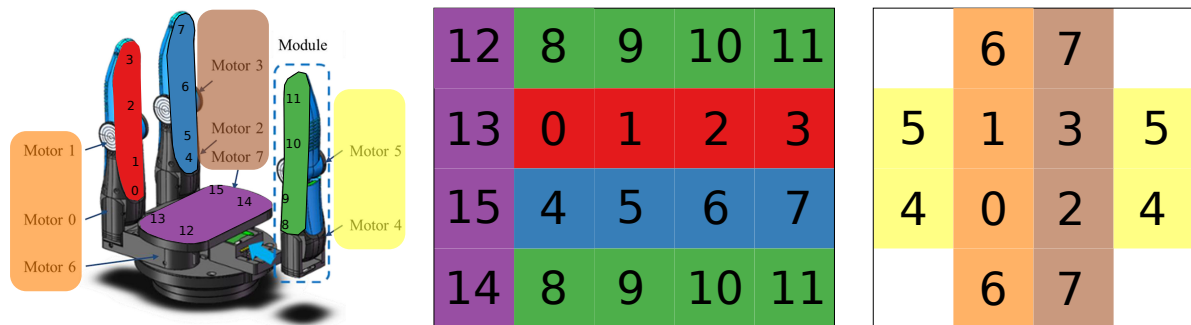
Figure 5.8: Left: Shoal hand (adapted from [8]) Middle: Arrangement of tactile sensor data in a 2D-grid to capture spatial relationships between sensors Right: Arrangement of joint motor positions in a 2D-grid to capture spatial relationships between the motors.
