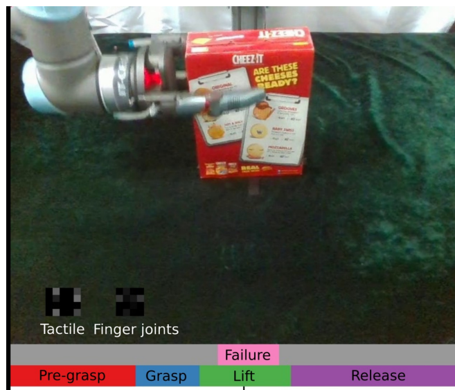
Figure 5.9: The temporal boundaries of the robot's actions in the VT dataset are annotated. We additionally annotate the start and end of the failure segments and represent the tactile sensor data and finger joint positions single channel images.
