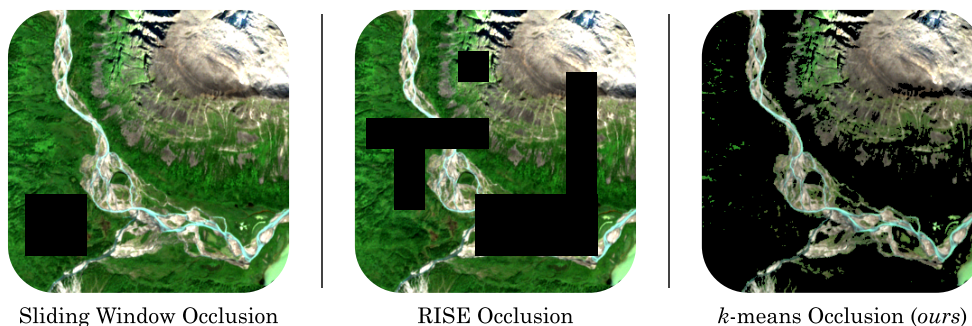
Figure 5.3: Sliding Window Occlusions by Zeiler and Fergus (2014) and RISE by Petsiuk et al. (2018) occlude the input using rectangular patches. In contrast, our Feature-specific Occlusion method simultaneously occludes similar feature vectors within the whole feature map. Although demonstrated here on an input image, our proposed method shows its true strength in the deep, intermediate layer of UH-Net, where the feature representations already correspond to meaningful concepts.
