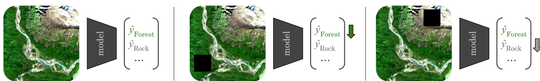
Figure 3.7: By systematically covering sections of a feature map (here the input image), one can observe how the model’s prediction changes, revealing the attributions of the occluded regions.
