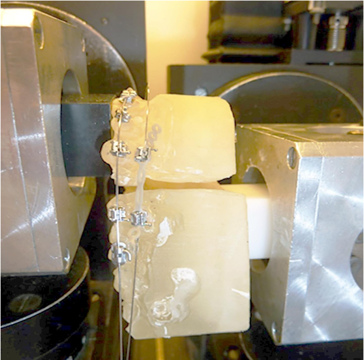
Figure 2: Frasaco model split up into an anterior and a posterior segment, mounted in the Orthodontic Measurement and Simulation System. The anterior segment is connected to the left force/torque transducer, the posterior to the right one. Simulated space closure is performed along the Z axis.
