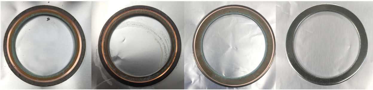
Figure 3.8: Overview of CF DN40 vacuum gaskets used in the experimental setup. The first three – cube towards source, main chamber IGP and gate valve – are gaskets used in the vacuum chamber for about 4.5 years being exposed to mercury vapor. They show green to dark gray colored corrosion along the vacuum sided edge of the gasket, that also leave a corrosive residue on the underlying aluminum foil. The corrosion on the outer air-sided edge stems from baking. The last gasket shows a chromium plated copper gasket tested in the rebuild of the vacuum chamber to prevent mercury corrosion.
