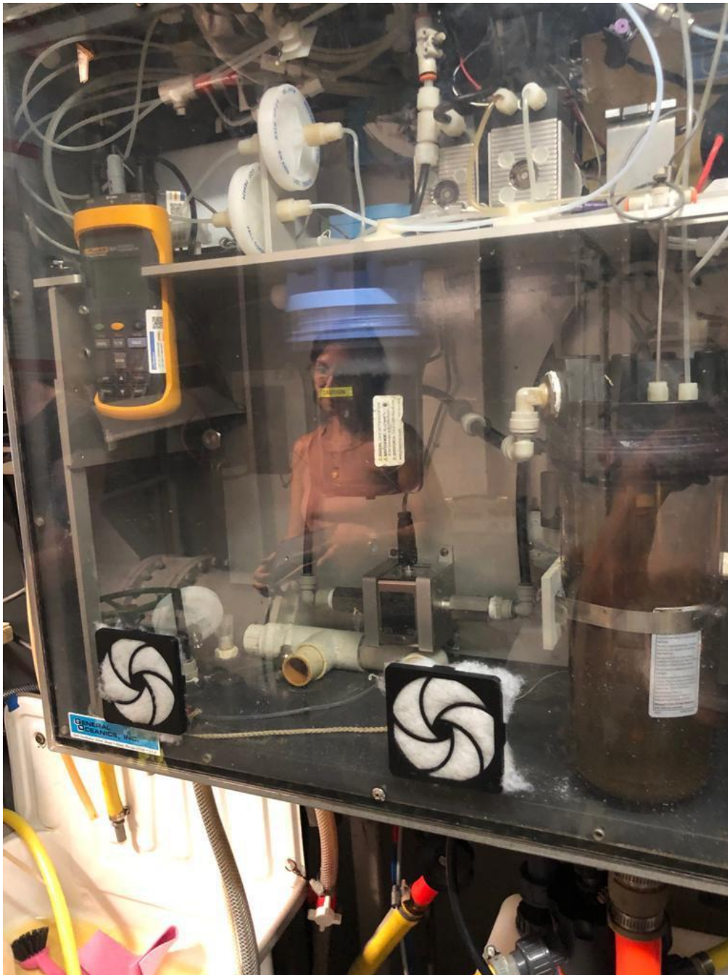
Picture 16: A reflection of myself while participating in the maintenance of an autonomous marine carbon observation system on a merchant vessel (a so-called Ship of opportunity (SOOP)) harbouring in Hamburg, Germany in 2022. Source: Mirja Schoderer.
