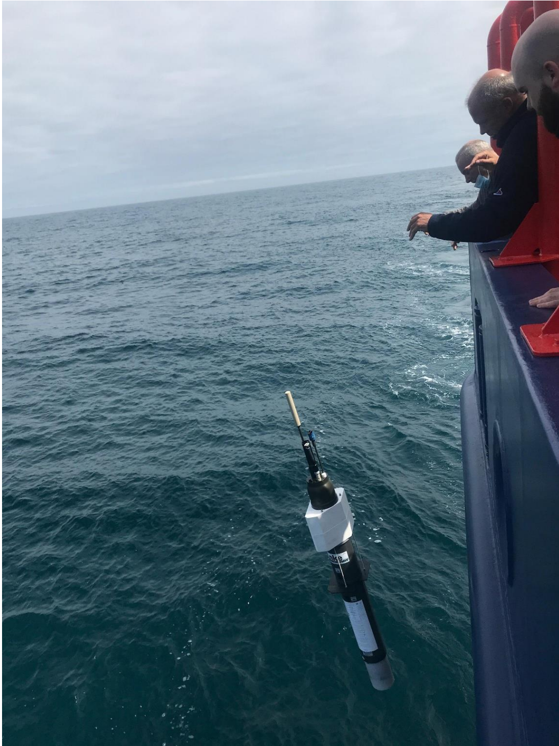
Picture 14: The deployment of an Argo float for MCOs from a German research vessel during an expedition in the North Atlantic in 2021. Source: Author.
