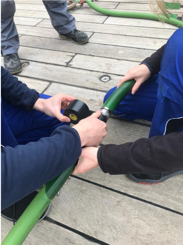
Picture 11: Repairing a defective part of the streamer, 31.07.2021. Source: Author.
