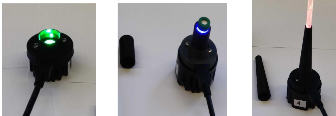
Figure S64. Pictures of the ex-situ illumination setup with USB-powered homemade light sources using commercial LED chips with 3D printed adaptors for 2 mL GC vials and 5 mm NMR-tubes.
