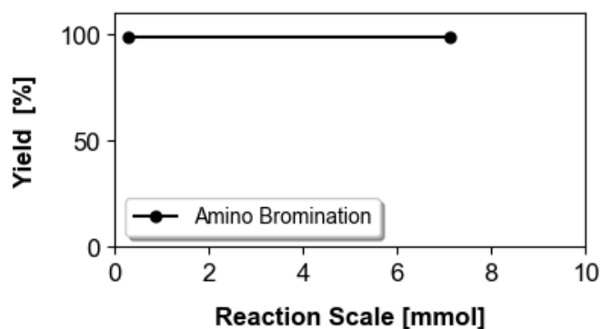
Figure S43. Plot of reaction scale in mmol against the isolated yield. Every data point represents an experimentally determined yield of I .
