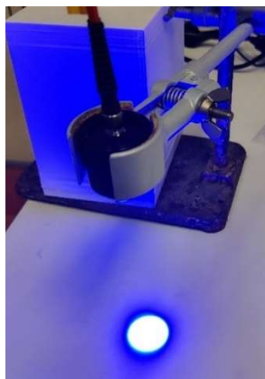
Figure S22. Irradiation setup with a collimator connected to the fibre collimated light source showing an evenly irradiated circle with a diameter of 4 cm. Samples were placed 2 cm under the collimator.
