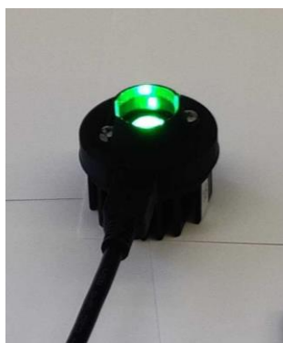
Figure S48. Pictures of the ex-situ illumination setup with USB-powered built-in-house light sources using commercial LED chips with 3D printed adaptors for 5 mm NMR-tubes.
