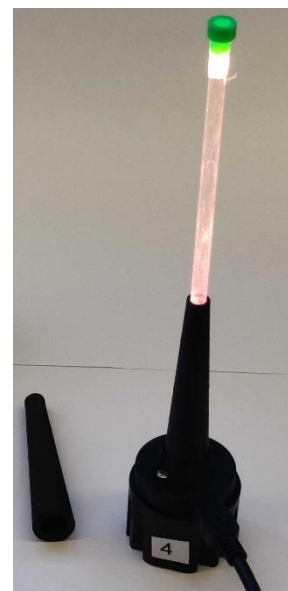
Figure S48. Pictures of the ex-situ illumination setup with USB-powered built-in-house light sources using commercial LED chips with 3D printed adaptors for 5 mm NMR-tubes.
