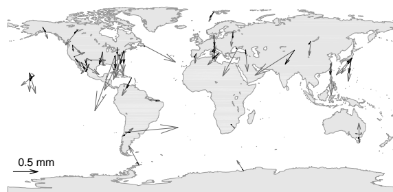
Fig. 5 Global map with mean values over 1990.0 - 2011.0 for total tropospheric gradients from solution 2 (light grey) and solution 3 (black). Plotted are stations that participated in more than 20 sessions.
