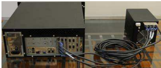
Fig. 2 Rear view of Mark 6 controller with disk module
