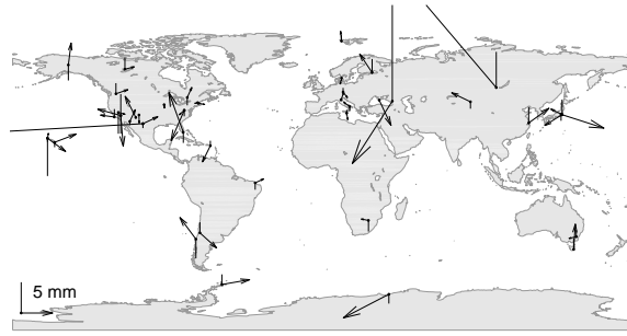
Fig. 2 Horizontal and vertical position differences at epoch 2000.0 between VieTRF10 and VTRF2008. Only differences for stations participating in more than 30 sessions are plotted.
