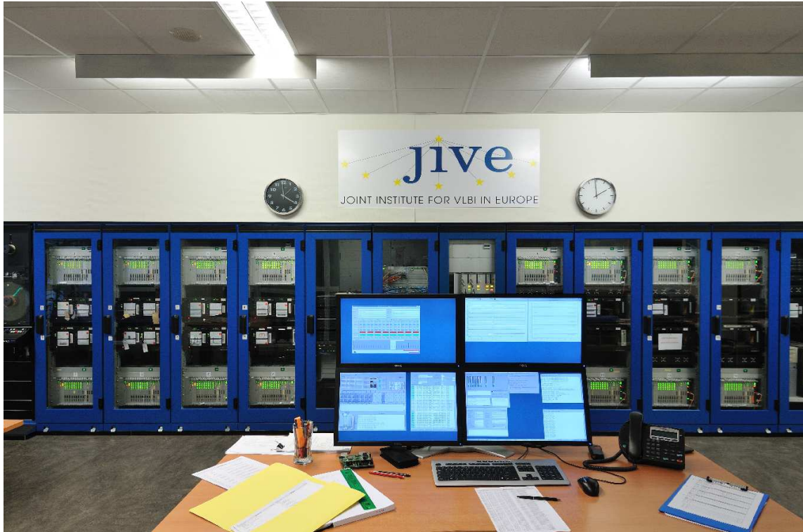
Fig. 1 The control station in the JIVE correlator room. The climate controlled row of racks in the background houses sixteen Mark5A or Mark5B units with corresponding stations units as well as the software FX correlator (central racks).
