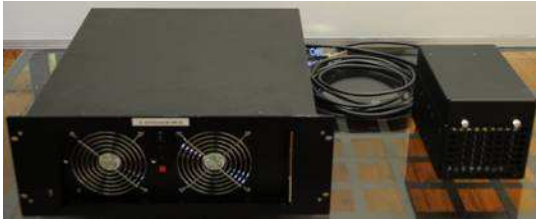
Fig. 1 Front view of Mark 6 controller with disk module
