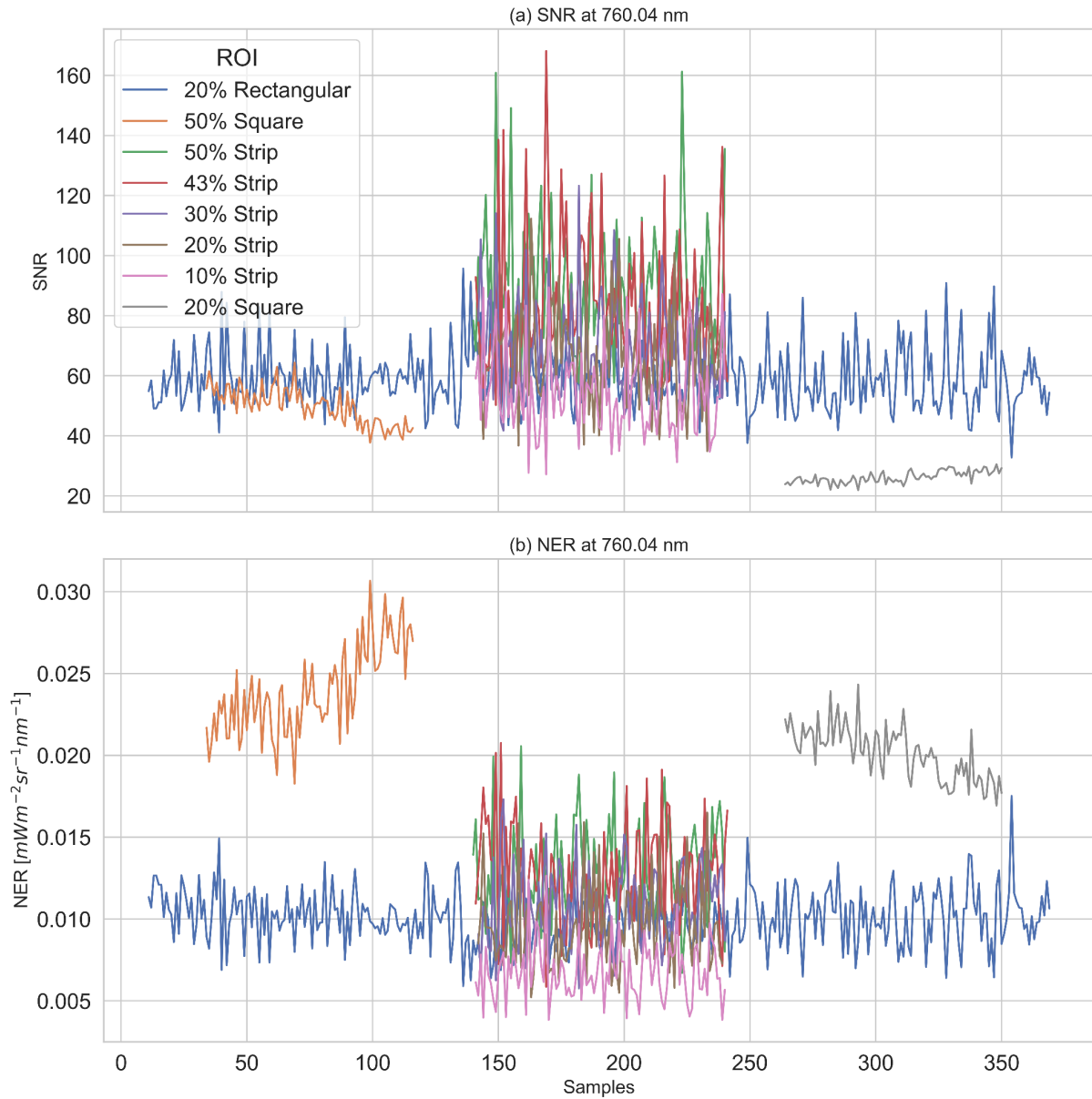
Figure 2.16 The sample-dependent signal-to-noise ratio (SNR) and corresponding noise-equivalent-radiance (NER) at the O 2 A band (760.04 nm) from four reference panels measured by HyScreen’s FLUO sensor.
