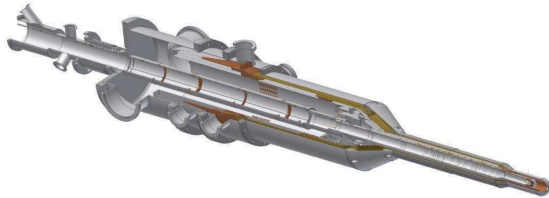
Figure 2.7: Bonn Frozen Spin Target: The actual target cell is located in the tip on the right [Wal07].
