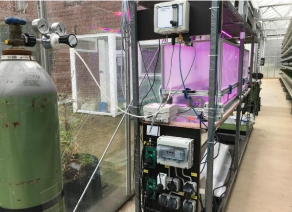
Fig.13: Open top growth box with independent temperature and CO 2 injection control.
