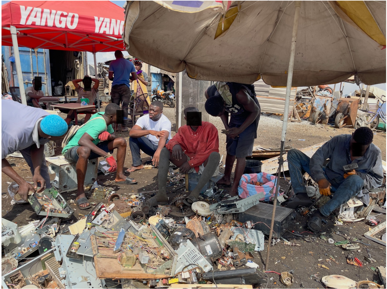
Figure 4. Manual dismantling of e-waste by workers. Source: Photograph by author, 2021.
