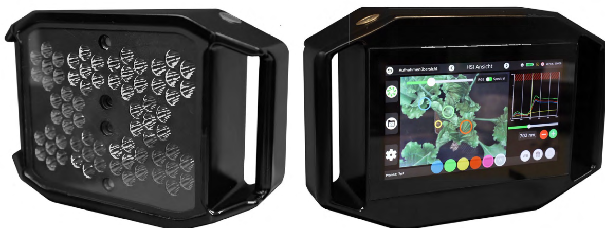
Fig. 2 Blackmobile front and back view. The frontside shows a 7" LED touchscreen that displays the user interface running the hypercube view widget. The backside shows the broadband VIS/NIR LED array, the lenses of the hyperspectral and RGB camera, and the laser system for vertical alignment
