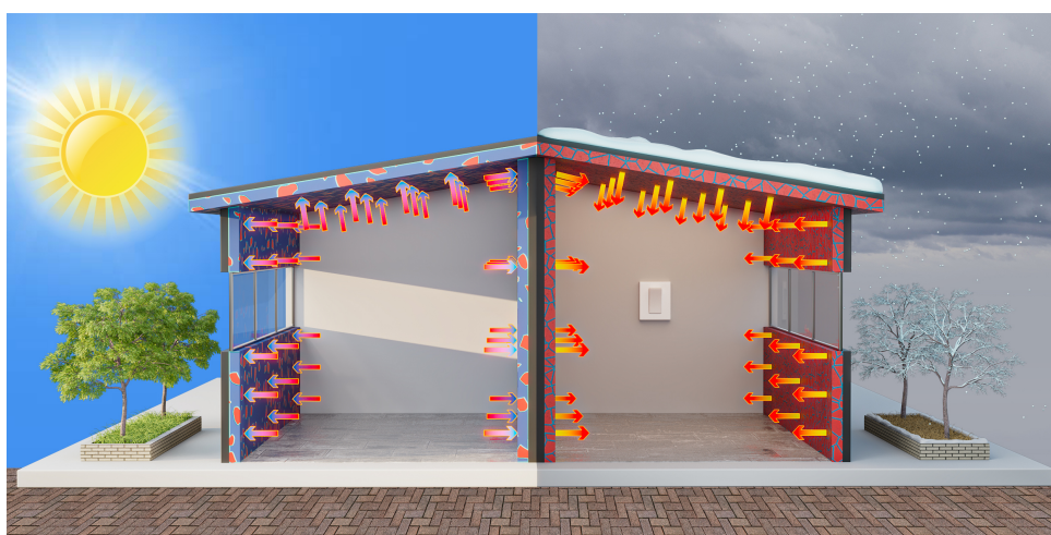
Figure 1.2: Proposed use of a heat-storage material integrated into the building materials of a structure, which can undergoes a phase transition during the warmer seasons (left) and releases the accumulated thermal energy on demand in winter (right).
