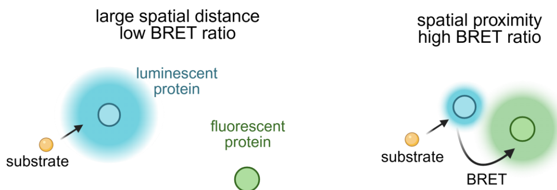
Figure 17: Principle of bioluminescence resonance energy transfer (BRET).
